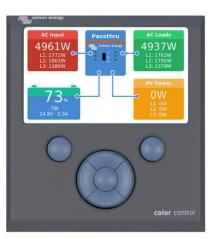
Color Control panel, showing a PV application
